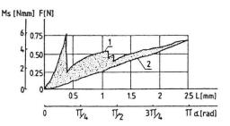
Fig. 2. Torsion curve of the pod: 1 - curve obtained in first torsion (intact pod), 2 - curve obtained in second torsion of the same pod,  $M_s$  - torque, F - registered force,  $\alpha$ - torsion angle, L - calculated linear deformation.
